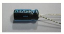
polarized or electrolytic capacitors are either marked similar to non-polarized caps if the body is real small or marked plainly on large body caps
